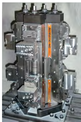
DUO 125 4 x 90° with special width-reduced jaws for 1st and 2nd clamping
