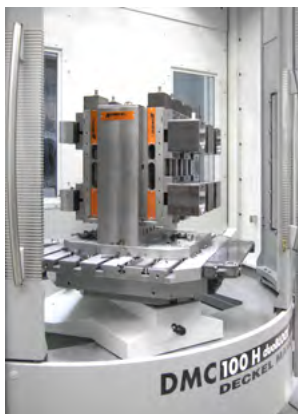
6-compartment design DUO 125 on double bracket
